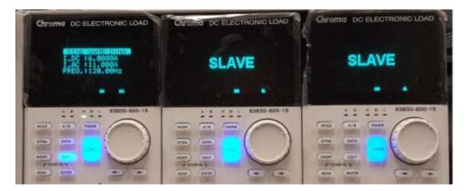
The above photo shows 3 63630-600-15 loads in parallel with the output voltage set to 75Vdc
